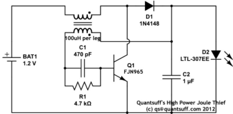
When power is applied, current flows from the battery through the diode, the resistor to the Base, starting the oscillation. After that, the LEDs act as a zener to maintain a relatively stable supply to the base.
