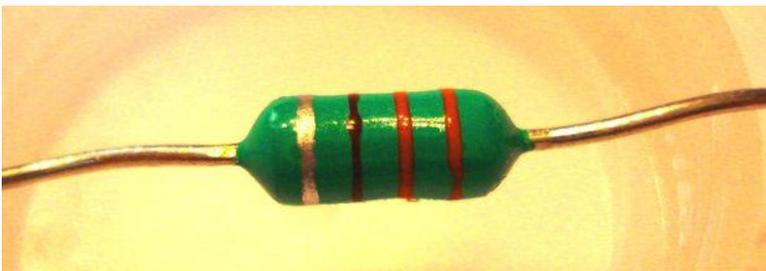
Although the IC "Joule Thief" seems to work with my crude, handwound coil on a nail, I actually use a very small 330 (orange-orange-brown) inductor that has the size and appearance of a small 1/2 watt resistor.
