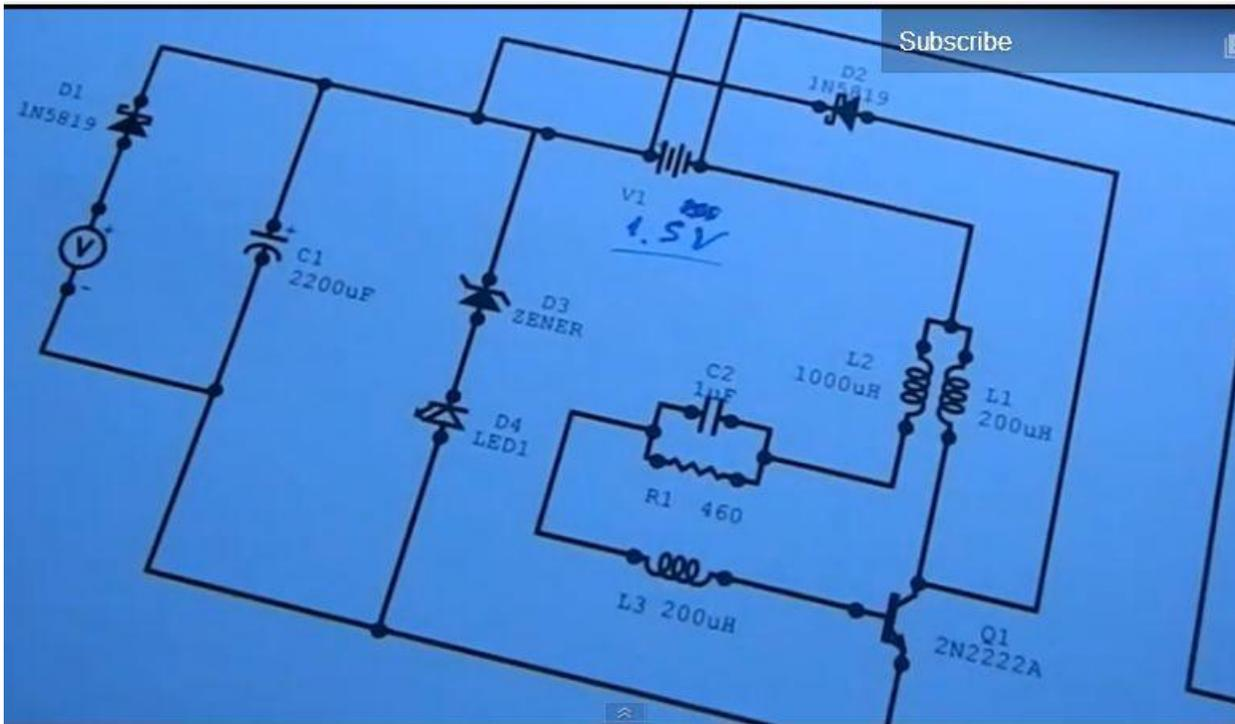
the battery in series with the coils. This is my first project using a solar panel and a charging joule thief without toroids or wounded air-coils. Using just inductors works very very nice. This circuit also uses a drive circuit shown later in video:
