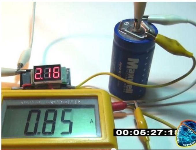
Above is supercap charging polarity. Charging wires are the two white wires. The bottom darker wire below is not a charging wire
