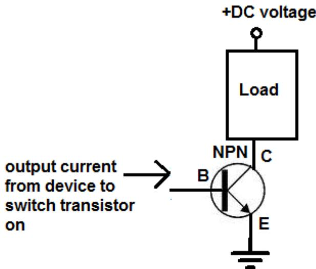
The output of the device that outputs a current will be connected to the base of the transistor. The load will be connected to the collector as well as the positive DC voltage for NPNs. The emitter will connect to ground.
