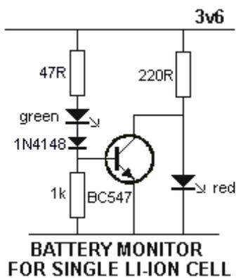
The following circuit monitors a single Li-ION cell. The green LED illuminates when the voltage is above 3.5v and the goes out when the voltage falls below 3.4v. The red LED then illuminates.
