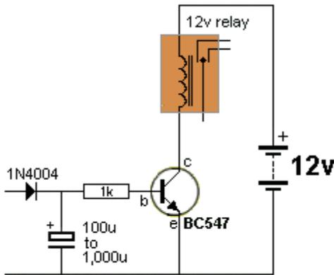
This circuit turns ON a relay when the input is above 2v (change resistor for more volts?) and the relay turns OFF after 2 seconds when the signal is removed. The OFF delay can be increased or decreased.
