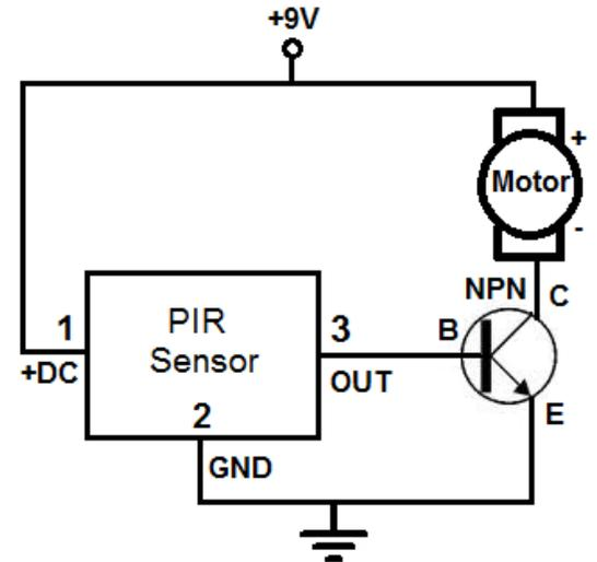
**Electronics Components: Use a Transistor as a Switch**
