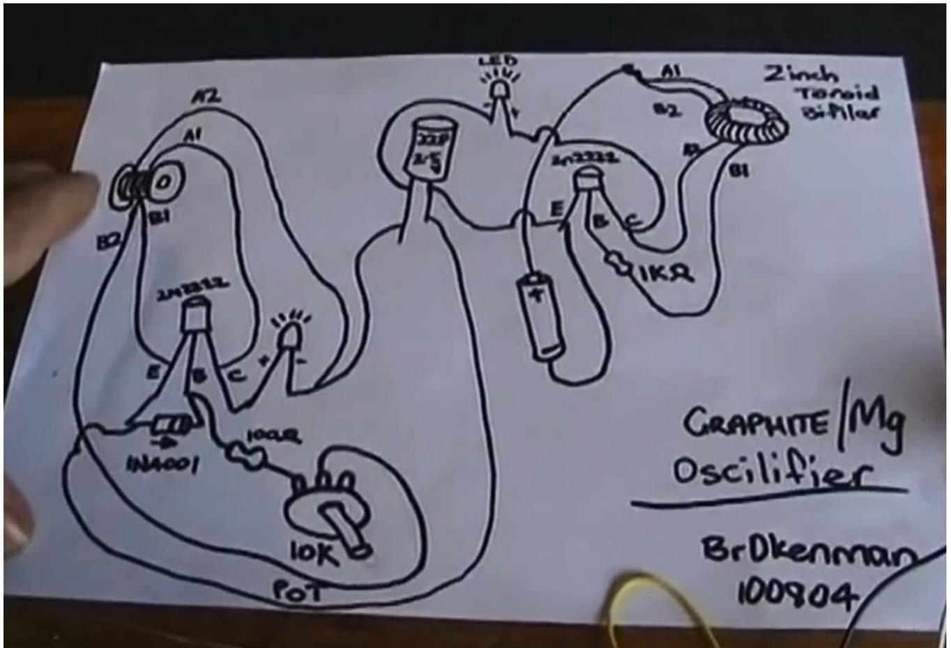
Upper Right hand of pic is the Joule Thief, which uses an LED as a Load (The LED was replaced with a 1N4004 Diode) the current then runs to a 22 farad 2.5 volt SuperCap
