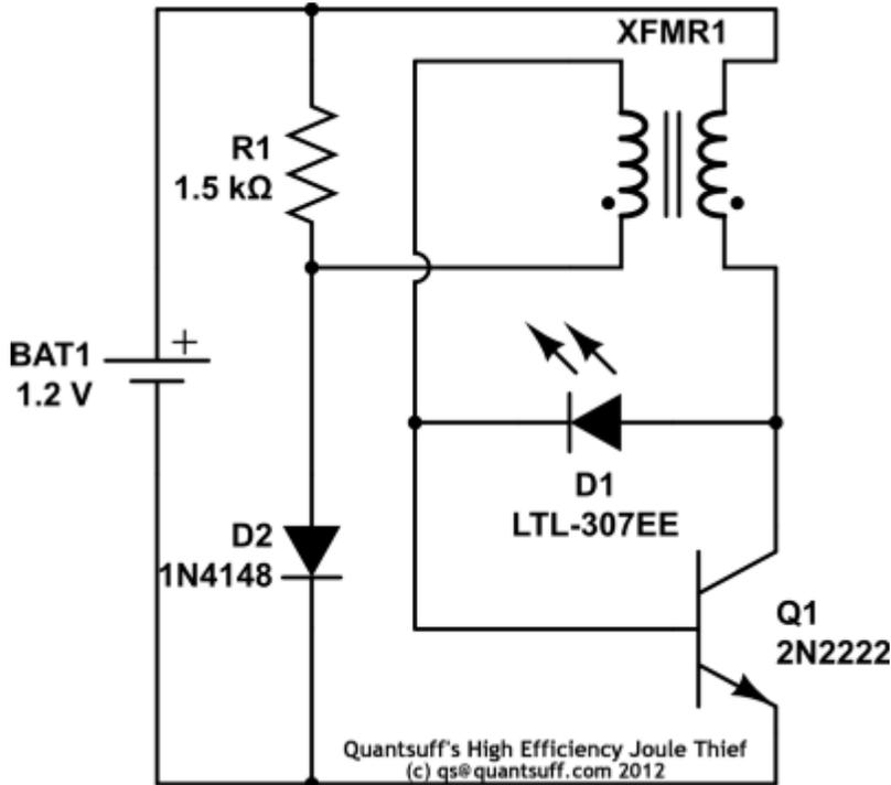
The addition of D2 represents an added drain of about 0.7mA, but aside from providing a return path to the LED, it also functions as a rudimentary power regulator by maintaining the voltage to the transistor's base just at its conducting point, regardless of input voltage. This allows the circuit to operate over a much wider voltage range, from 2-volts to around 0.9-volt with much better current (and brightness) regulation. As built, this circuit will operate down to just below 0.6v.
