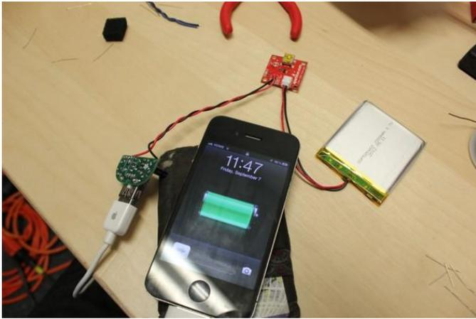
In under two hours, I had gotten most of the way there, and just need to attach the solar panel and cut out the Altoids case.
