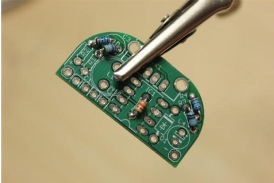
[Enlarge](#) / The MintyBoost, once I had soldered on all the resistors.
